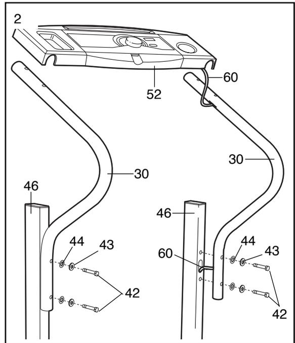
3. Attach the Console Base (52) to the Handrails (30) with four Handrail Screws (11).
