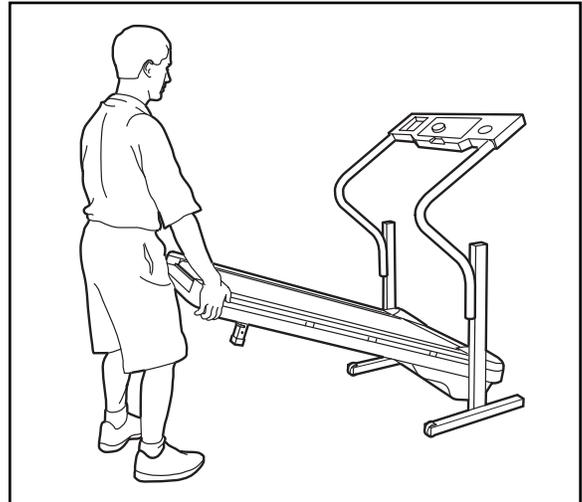
2. Move your right hand to the position shown and hold the treadmill firmly. Using your left thumb, press the storage latch and hold it. Pivot the treadmill until the frame and foot rail are past the storage latch. Close the storage latch over the catch. **Make sure that the storage latch is fully engaged over the catch.**
