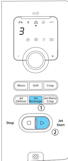
**THE JET BEVERAGE FUNCTION PROVIDES** you with an easy way to quickly reheat 1-4 cups of beverage.
