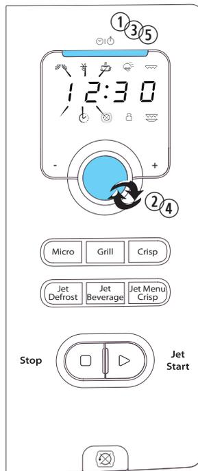
**WHEN THE APPLIANCE IS FIRST PLUGGED IN** or after a power failure, it will enter clock setting mode automatically.
