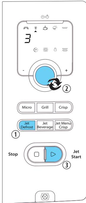
**USE THIS FUNCTION** for defrosting Meat, Poultry, Fish, Vegetables and Bread. JET Defrost should only be used if the net weight is between 100 g- 2.5 kg.
