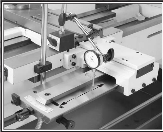
**Figure 20. Taper attachment alignment.**
