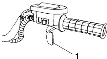
This ATV is equipped with Polaris Electronic Throttle Control (ETC), which is designed to reduce the risk of a frozen or stuck throttle. If the throttle cable should stick in an open position when the operator releases the throttle lever, the engine will stop, and power to the rear wheels will cease.
