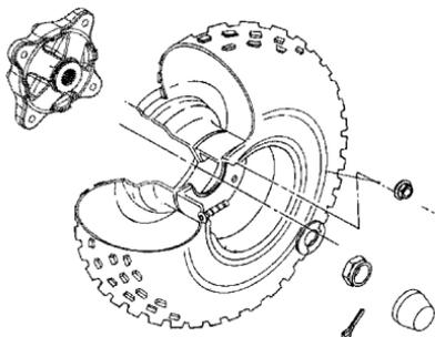
2. Place the wheel on the wheel hub with the valve stem toward the outside and the rotation arrows on the tire pointing toward forward rotation.
