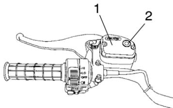
**NOTE:** When checking the fluid level, the ATV must be on level ground with the handlebars straight. If the fluid level is low add DOT 3 brake fluid only. See page 114 for the part numbers of Polaris products.
