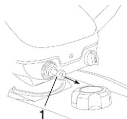
**NOTE:** The variable choke is fully on when the knob is pulled completely out. The choke is off when the knob is pushed completely in. The choke can be adjusted gradually, depending on how much choke is needed for starting. Be sure the choke is off during operation, as excess fuel washing into the engine oil will increase wear on engine components.
