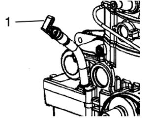
**NOTE:** Lift the lever lock (2) to remove the dipstick.
