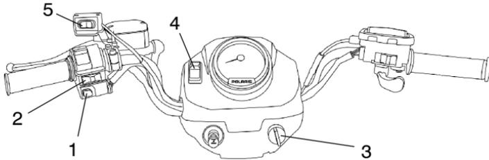
**Mode/Reverse Override Switch (1)** - This vehicle is equipped with a reverse speed limiter system. To gain additional power while backing, depress the override switch.
