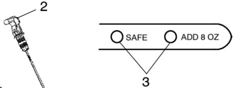
**NOTE:** Due to the dipstick entry angle into the crankcase, the oil level will read higher on the bottom side of the dipstick. Always read the level on the *upper* surface (4) of the dipstick.
