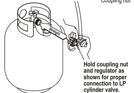
6. Turn the coupling nut clockwise and tighten to a full stop. The regulator will seal on the back-check feature in the LP cylinder valve, resulting in some resistance. **An additional one-half to three-quarters turn is required to complete the connection. Tighten by hand only – do not use tools.**
