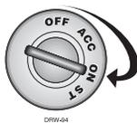
To disarm the security system, turn the ignition key on and press the Valet switch within 15 seconds. The system should now disarm. If the system does not disarm, you may
