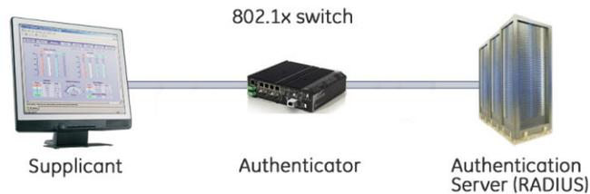
**FIGURE 7-1: 802.1x network components**
