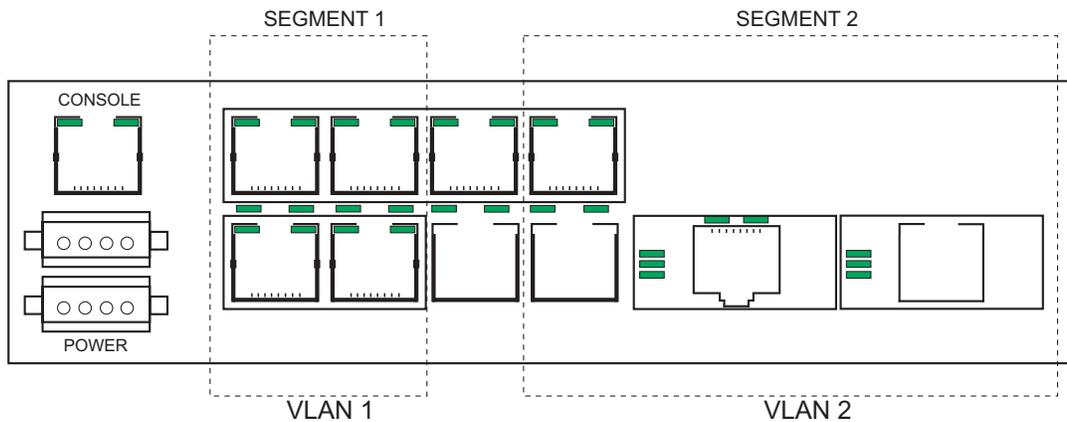
**FIGURE 10-1: VLAN as two separate broadcast domains**
