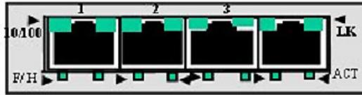
The ML1200's 4-port Copper module, the C1 Module, provides four 10/100Mb switched RJ-45 ports. The 10/100Mb switched ports normally (as a default setting) are independently N-way auto-negotiating and auto-crossover (MDIX) for operation at 10 or 100Mb speed in full- or half-duplex mode. (i.e., each independently selects a mode and speed to match the device at the other end of the twisted pair cable).
