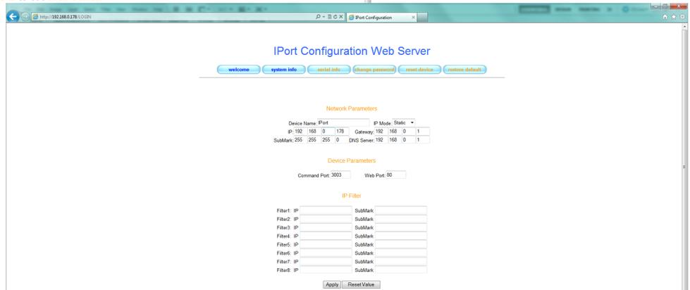
Change the IP on the computer from 192.168.0.80 to 192.168.1.80 then type the 192.168.1.178 into the address bar. If successful the log in page will display again.
