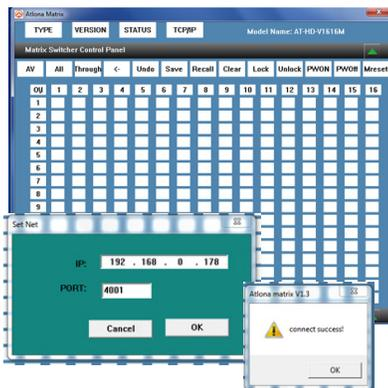
Once in the control interface there, click the TCP/IP button on the top of the window. Enter in the IP: 192.168.0.178 (192.168.1.178 if changed) and port 4001, if it has not already been auto-generated. If done correctly then a pop up window will display saying "connect success!".
