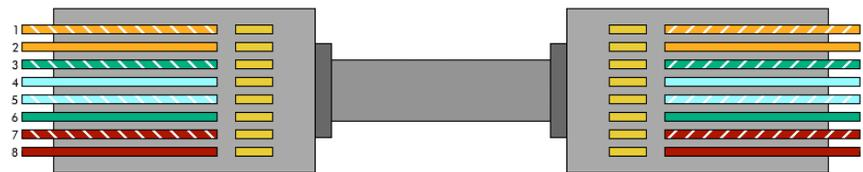
Use a straight cable to connect to a router or network.
