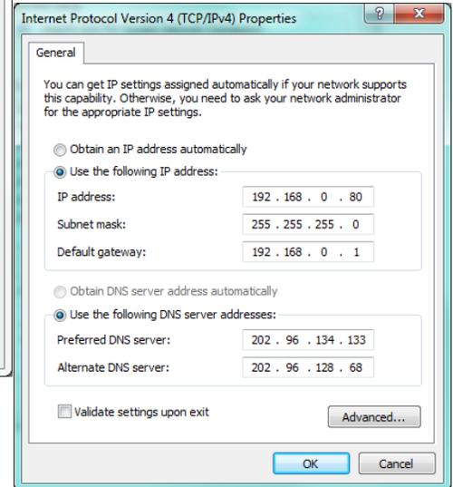
Once the window comes up enter in the IP address, subnet mask, default gateway, preferred DNS server and alternate DNS server information into each field.
