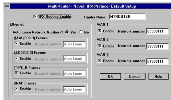
If your network protocol is **IPX**, continue with the following steps. If your network protocol is **IP**, click on the **IPX Routing Enable** check box to disable IPX, then click on the **OK** button and proceed to step 14.
