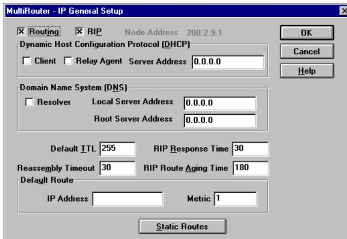
The IP General Setup dialog box controls the timers, DHCP (dynamic Host Configuration Protocol) and Domain Name System (DNS) servers, the default route, filters, and Static Routes.
