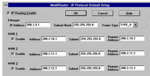
15. To change the IP parameters, proceed to the next step. Clicking on the **OK** button advances to the WAN Ports Default Setup dialog box. The WAN Ports Default Setup starts at step 20.
