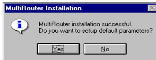
8. Ensure that the **Fail** LED is off before you click on the **Yes** button. Click on **Yes** to set up the default parameters. If you click on **No**, the installation is complete.
