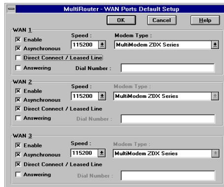
21. The **WAN** Ports Default Setup dialog box is displayed with all the WAN Ports enabled, Asynchronous mode enabled, the speed set at 115200, and the Modem Type defaulted to Socket Modem K56flex. Each WAN port can be configured independently; e.g., one can dial a specific number, another could answer a call, and the third could dial a different number.
