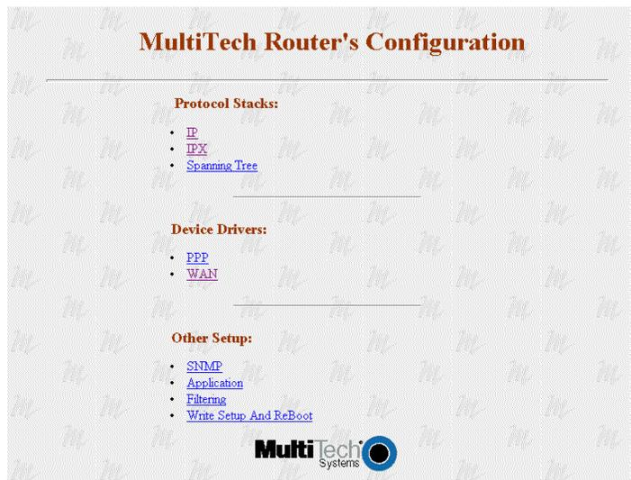
**Note:** The first user to access the RASFinder will have *read/write* rights over the unit. All subsequent users will have *read only* rights, and therefore, some of the options within the WEB interface will be inactive (i.e., will not be linked).
