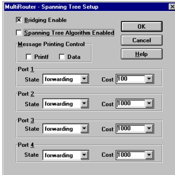
With Spanning Tree bridging, the RASFinder defaults with one logical WAN port mapped to a DLCI and set for “forwarding.” Any other WAN ports should be set for “blocking.” When it is required, the RASFinder will make the transition from blocking to forwarding automatically.
