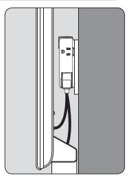
**Connect Your Surge Suppressor to the AC Power Line:** Plug the surge suppressor directly into a 3-wire grounded, 120V AC outlet.
