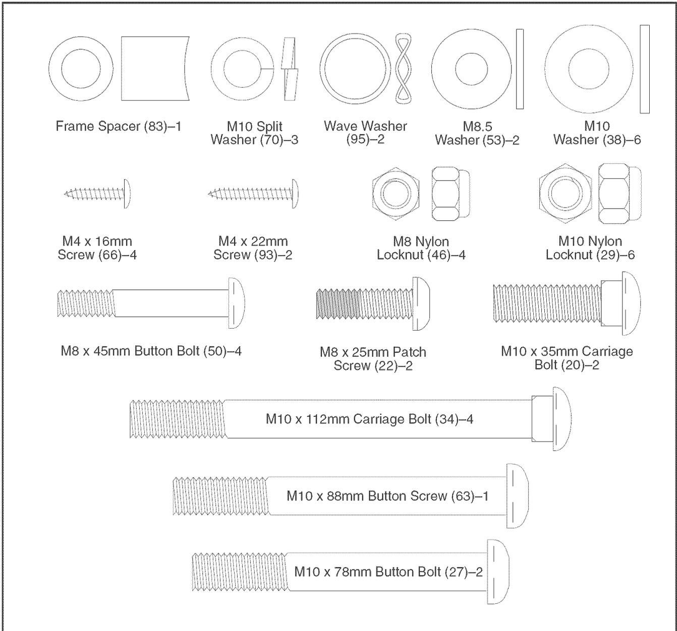
1. Identify the Front Stabilizer (3). While another person lifts the front of the Frame (1), attach the Front Stabilizer to the Frame with two M10 x 112mm Carriage Bolts (34) and two M10 Nylon Locknuts (29). **Make sure that the Front Stabilizer is turned so the Wheels (32) are not touching the floor.**
