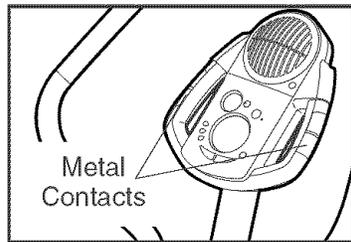
For the most accurate heart rate reading, continue to hold the handgrips for about 30 seconds. Note: When you first hold the handgrips, the large display will show your heart rate continuously for 30 seconds. The display will then show your heart rate along with other feedback modes.
