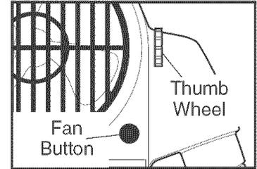
Rotate the thumb wheel on the right side of the console to pivot the fan to the desired angle.
