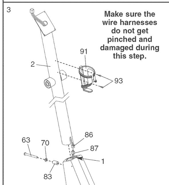
Slide an M10 Split Washer (70) and a Frame Spacer (83) onto an M10 x 88mm Button Screw (63). Insert the Button Bolt into the Frame (1) and the Upright (2). **Make sure that the concave end of the Frame Spacer is turned toward the Frame. Do not tighten the Button Bolt yet.**
