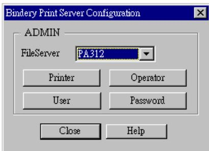
**Figure 14: Configure NetWare Server (Bindery PS mode)**
