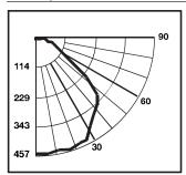
Test No. 11870.0 **H2601** Lamp=100WA19 Lumens=1750 Spacing Criteria=1.3 Efficiency=60.7%
