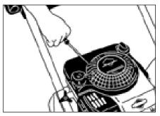
Step 6 Pull the starter handle. If the engine fails to start after 3 pulls squeeze the trigger gun to release pressure, and repeat step 7.
