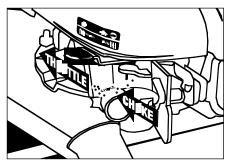
Step 5 Slide the throttle control to the fast position.
