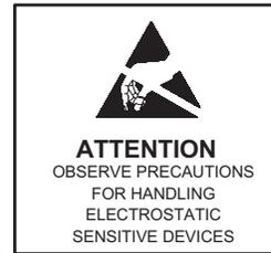
**WARNING: Electrostatic-sensitive device. Use proper CMOS/MOSFET handling precautions to avoid electrostatic discharge.**
