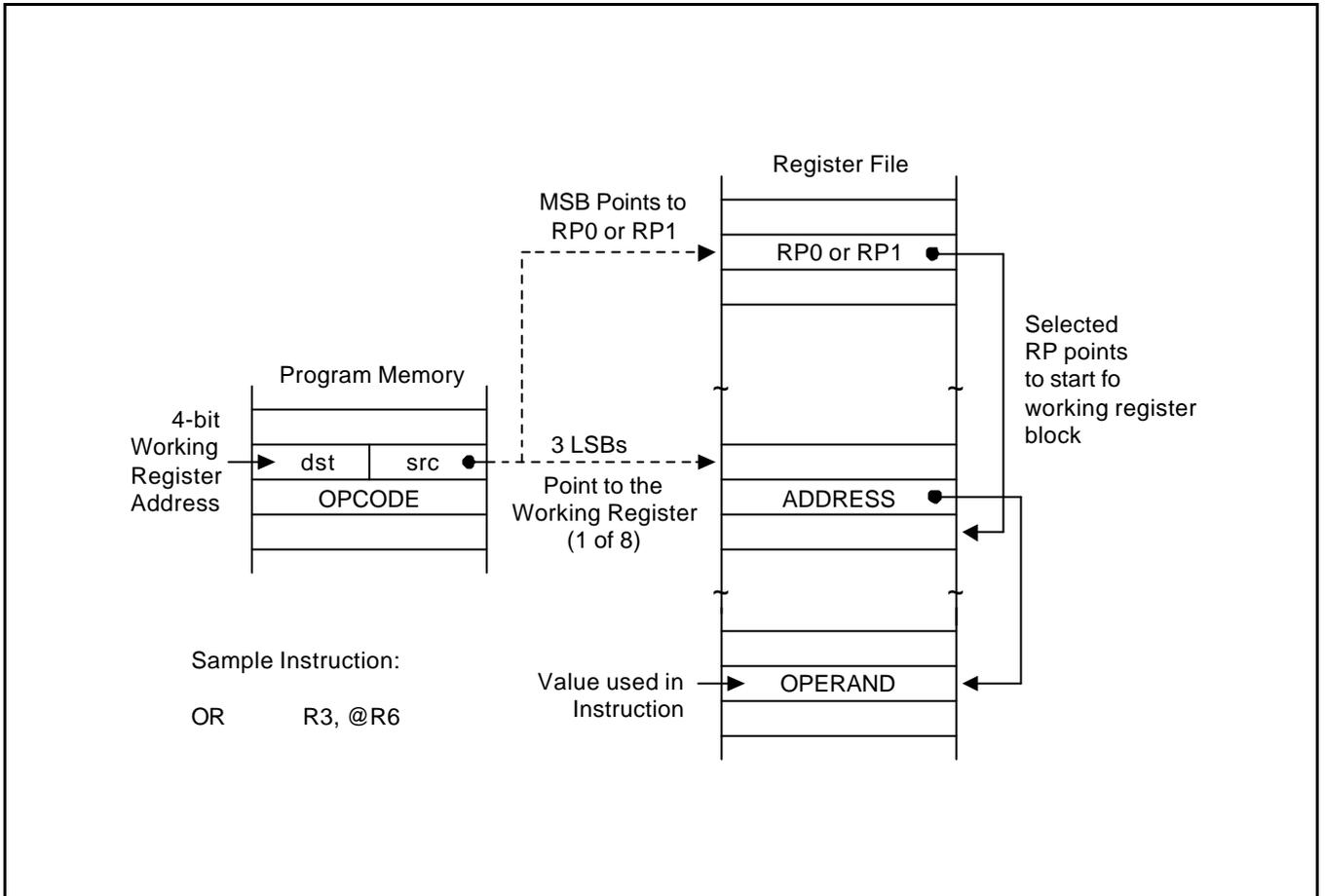
Figure 3-5. Indirect Working Register Addressing to Register File
