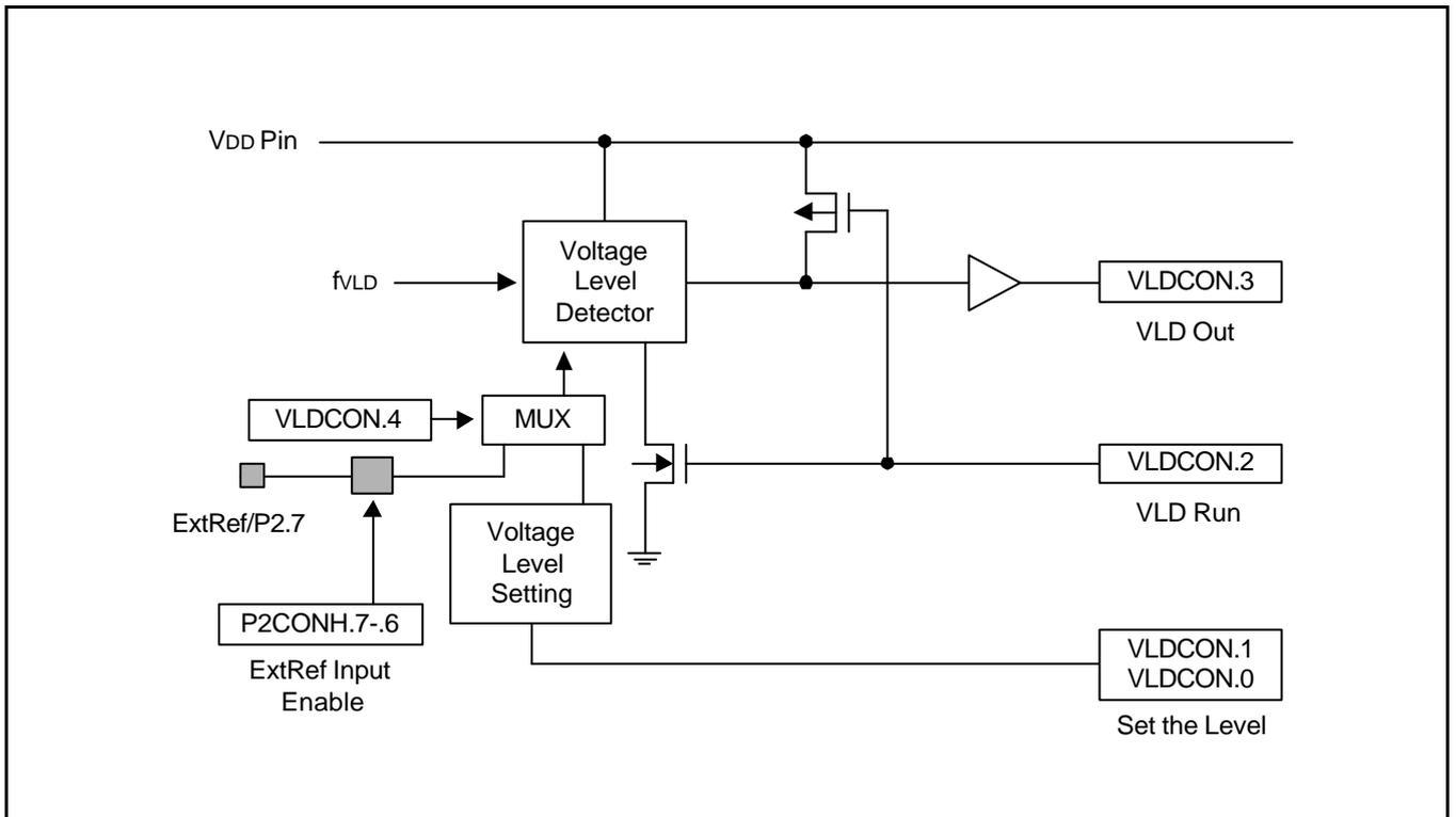
Figure 18-1. Block Diagram for Voltage Level Detect
