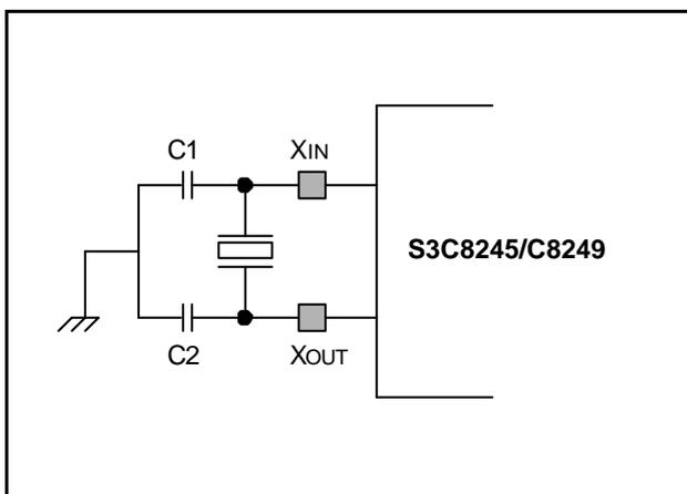
Figure 7-1. Main Oscillator Circuit
