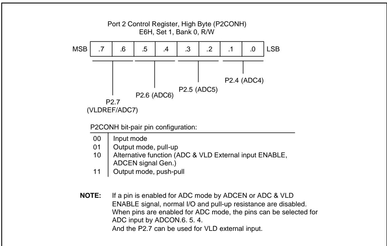
**Figure 9-8. Port 2 High-Byte Control Register (P2CONH)**
