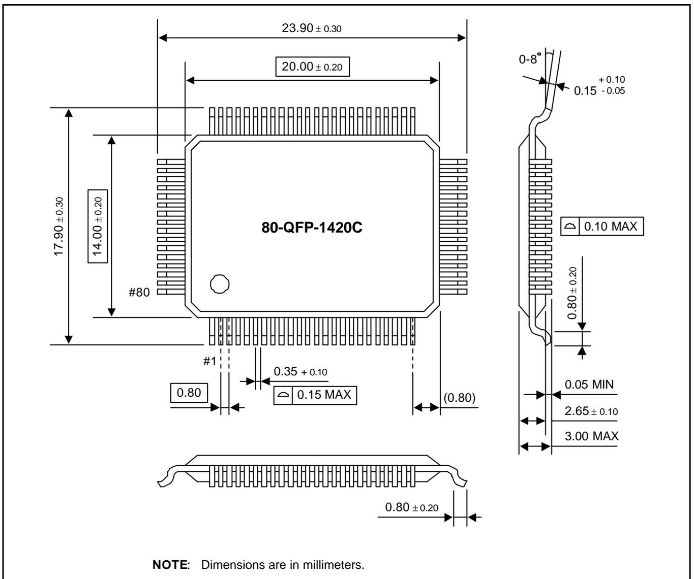
Figure 20-1. Package Dimensions (80-QFP-1420C)
