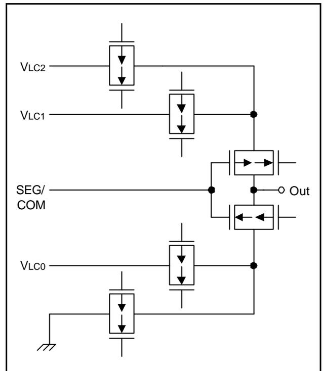
Figure 1-11. Pin Circuit Type H (SEG/COM)
