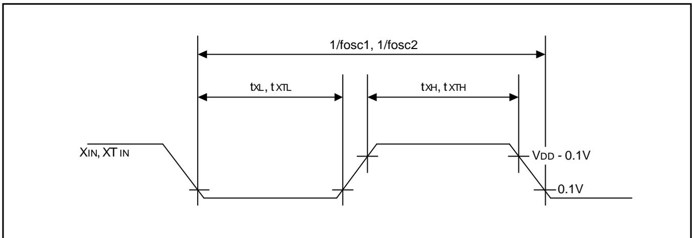
Figure 19-7. Clock Timing Measurement at  $X_{IN}$ Table 19-13. Sub Oscillator Frequency ( $f_{OSC2}$ )
