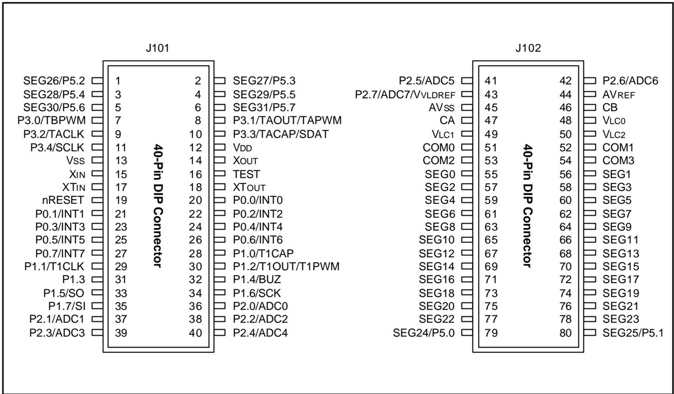
Figure 22-3. 40-Pin Connectors (J101, J102) for TB8245/8249
