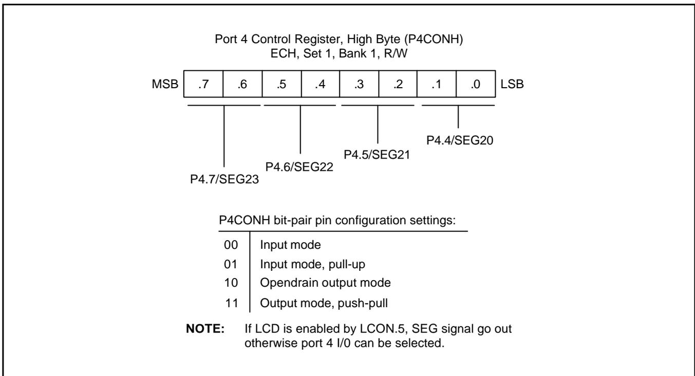
Figure 9-12. Port 4 High-Byte Control Register (P4CONH)
