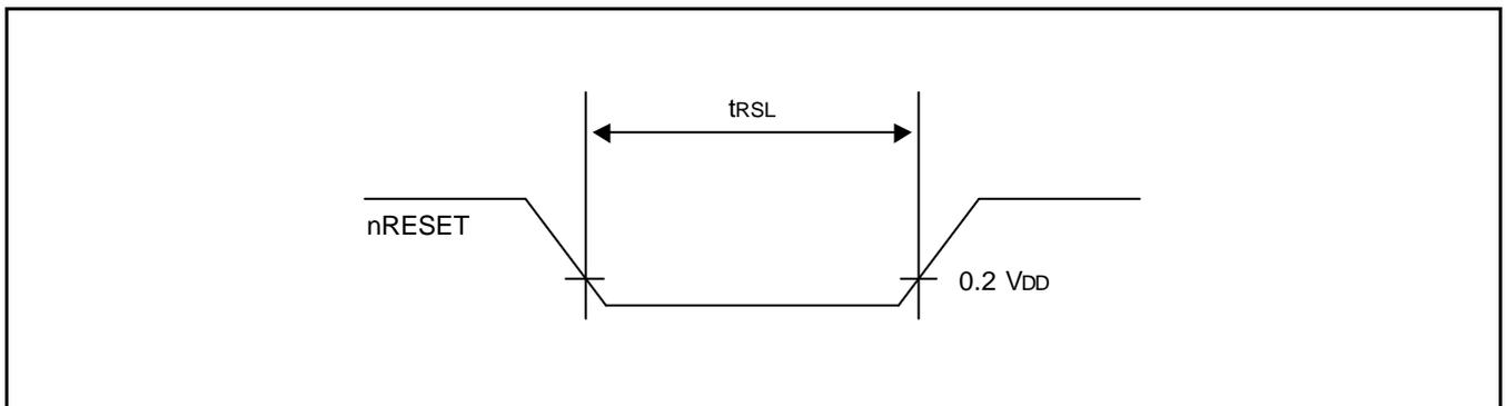
Figure 19-2. Input Timing for nRESET
