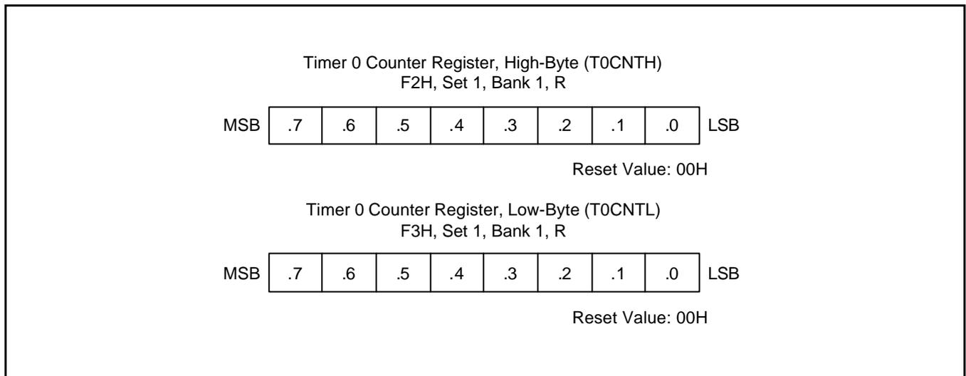
**Figure 12-3. Timer 0 Counter Register (T0CNTH/L)**
