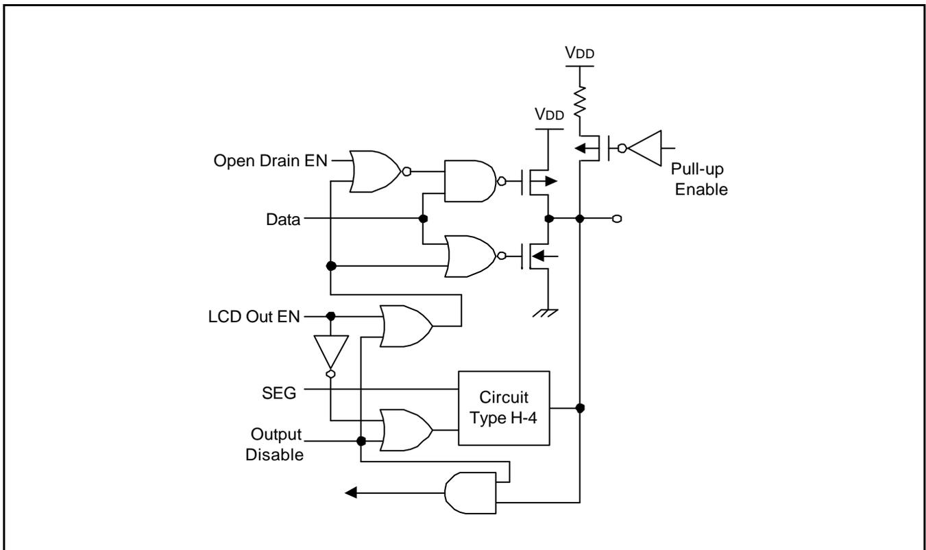
Figure 1-13. Pin Circuit Type H-14 (P4, P5)
