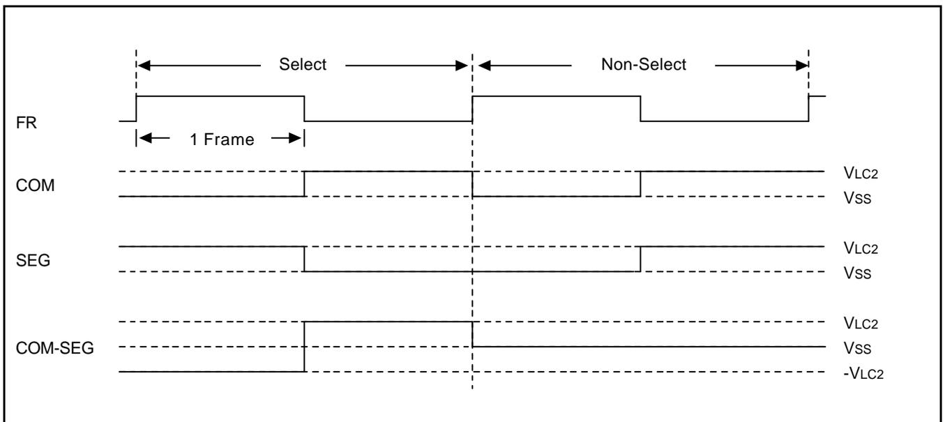
**Figure 14-4. Select/No-Select Bias Signals in Static Display Mode**
