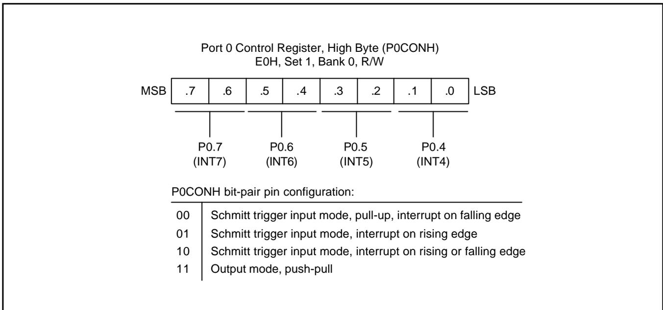
Figure 9-1. Port 0 High-Byte Control Register (P0CONH)
