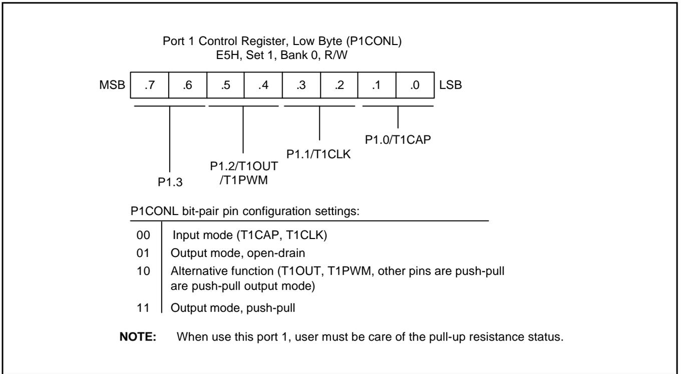
**Figure 9-6. Port 1 Low-Byte Control Register (P1CONL)**
