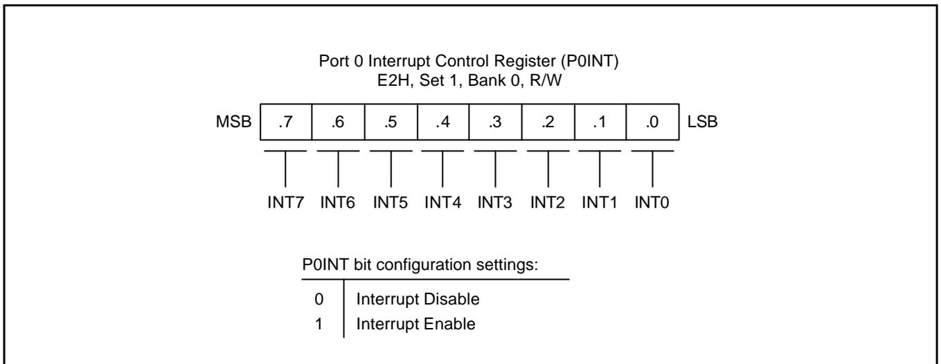
Figure 9-3. Port 0 Interrupt Control Register (P0INT)
