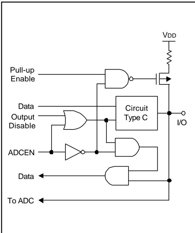
Figure 1-9. Pin Circuit Type F-10 (P2.0-P2.6)
