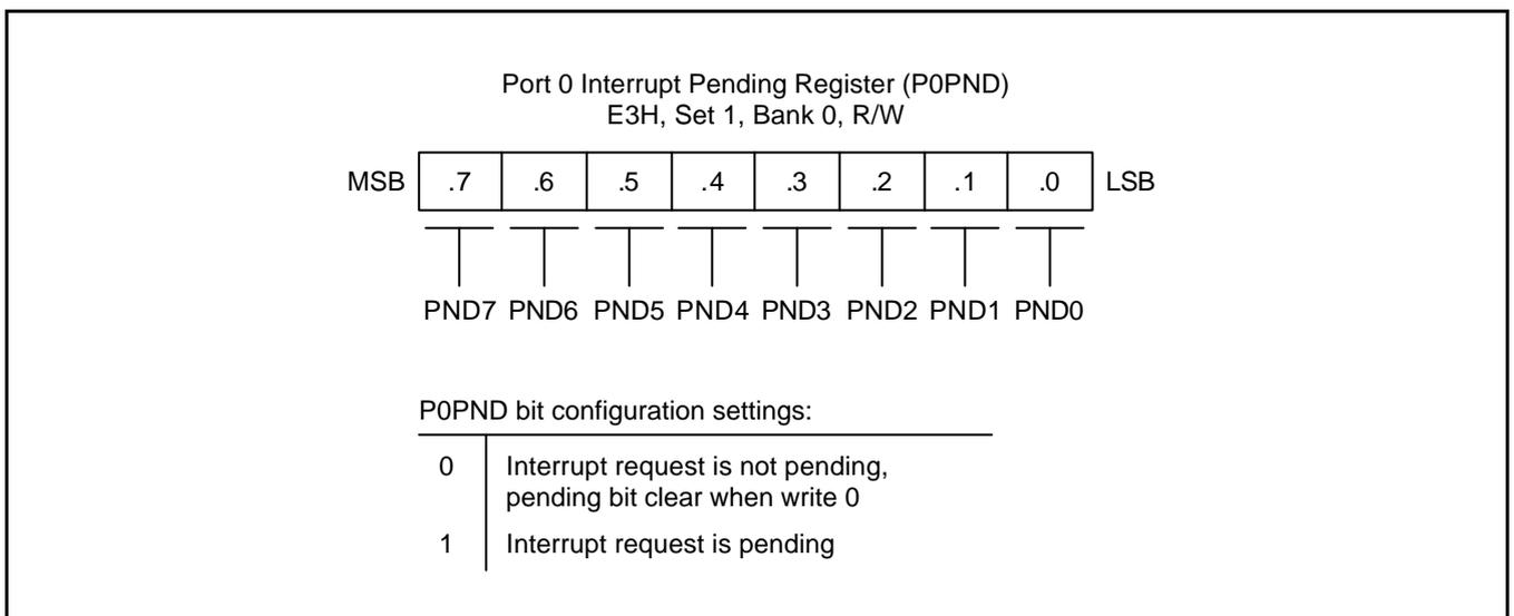
Figure 9-4. Port 0 Interrupt Pending Register (P0PND)
