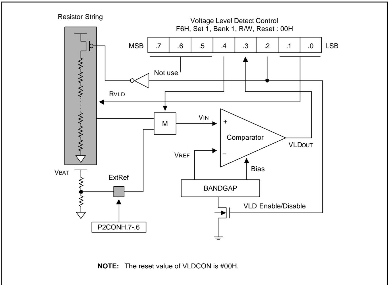
Figure 18-2. Voltage Level Detect Circuit and Control Register
