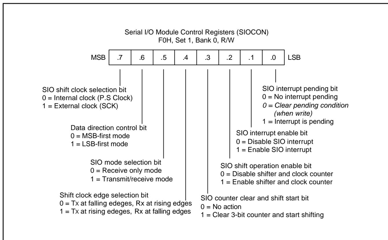
**Figure 16-1. Serial I/O Module Control Registers (SIOCON)**
