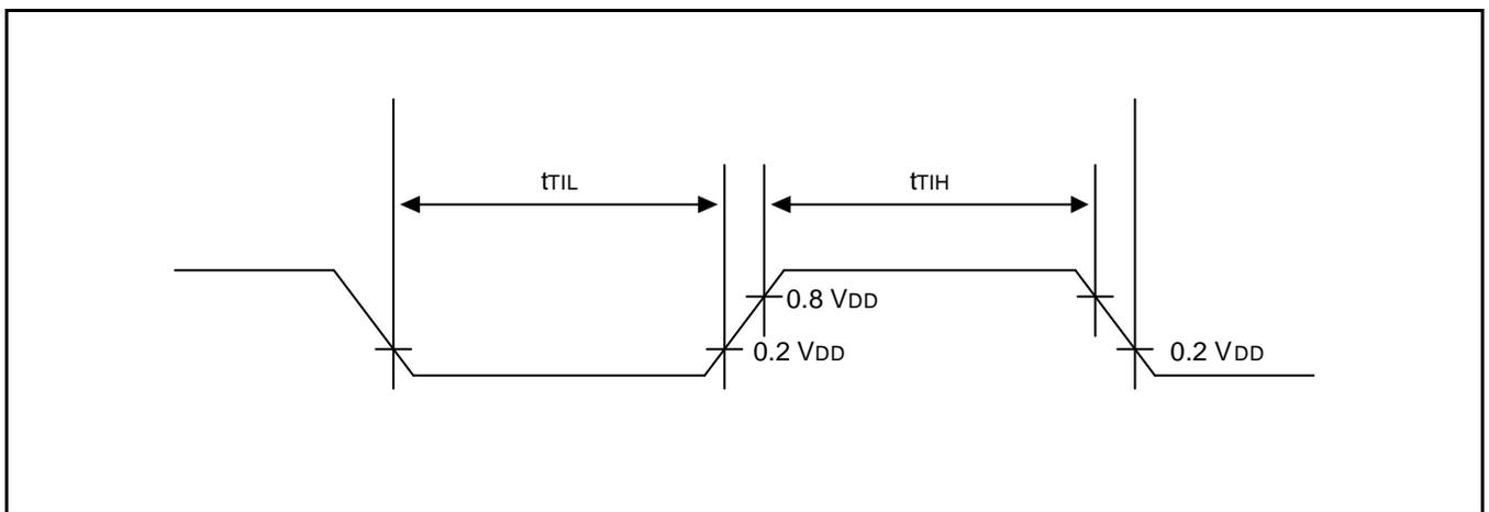
Figure 19-1. Input Timing for External Interrupts (Ports 0)
