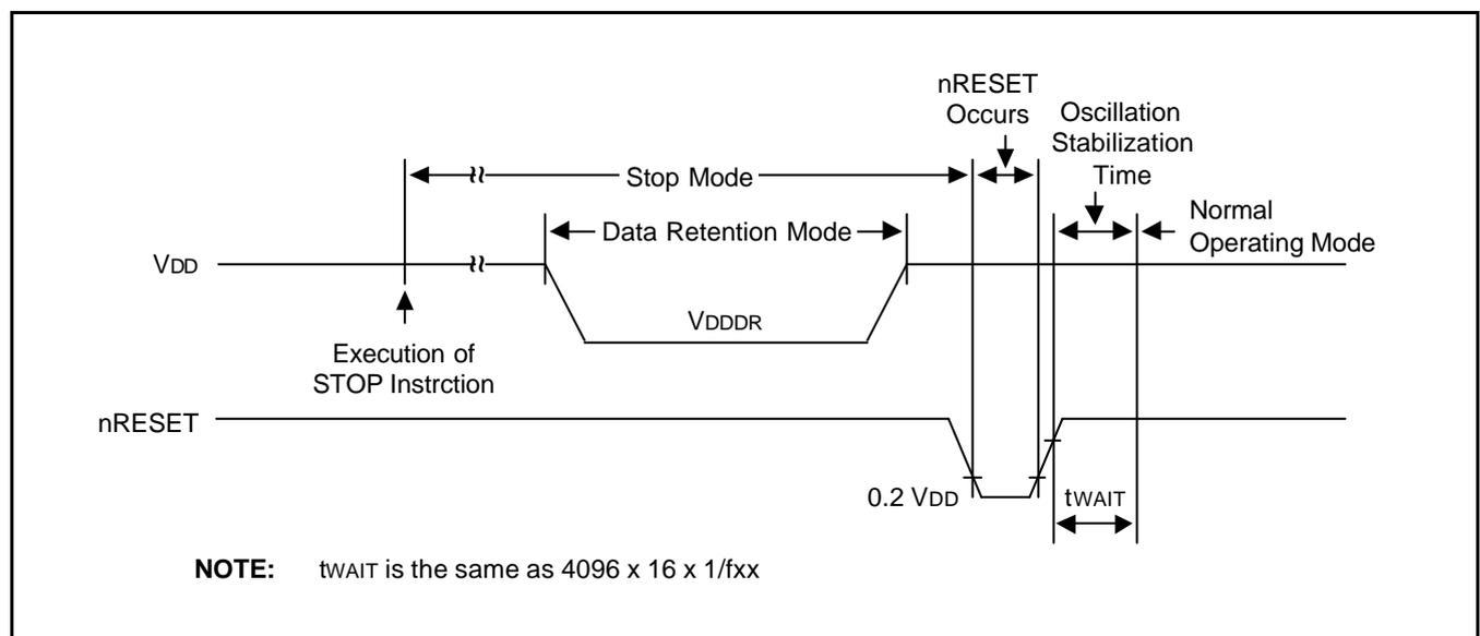
Figure 19-3. Stop Mode Release Timing Initiated by nRESET
