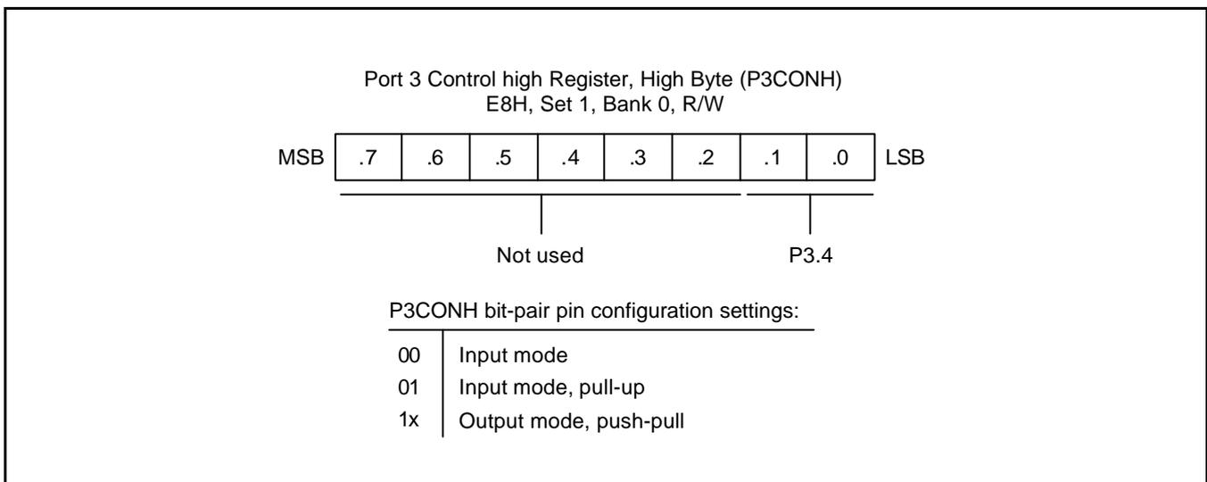
**Figure 9-10. Port 3 High-Byte Control Register (P3CONH)**
