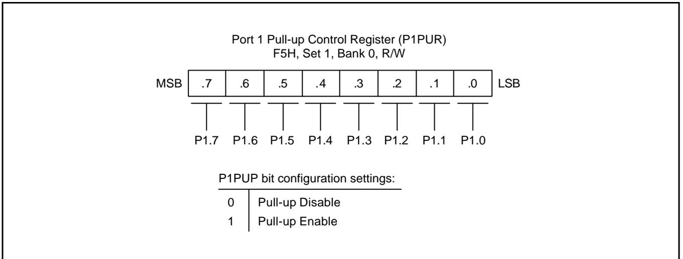
**Figure 9-7. Port 1 Pull-up Control Register (P1PUP)**
