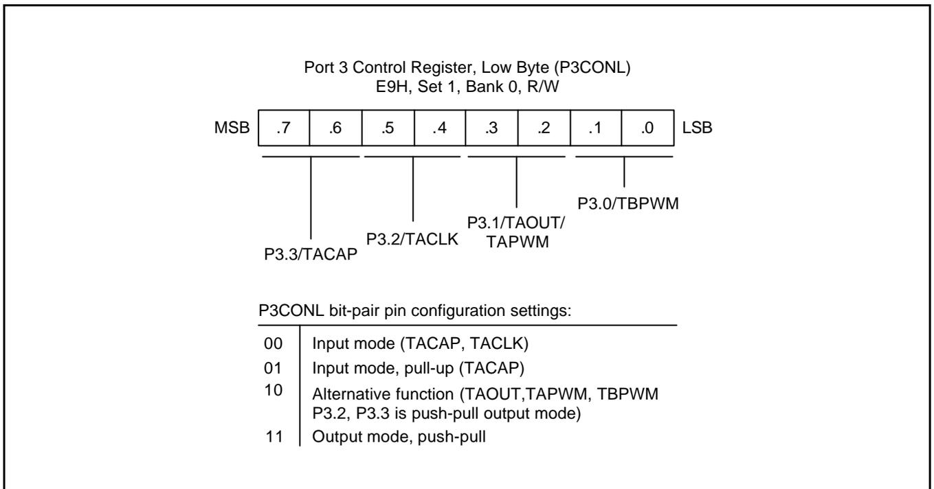
**Figure 9-11. Port 3 Low-Byte Control Register (P3CONL)**
