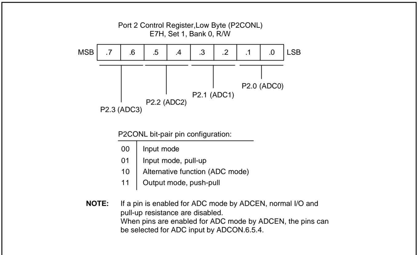
**Figure 9-9. Port 2 Low-Byte Control Register (P2CONL)**
