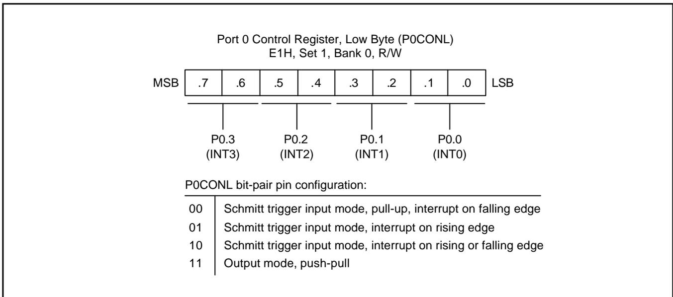
Figure 9-2. Port 0 Low-Byte Control Register (P0CONL)
