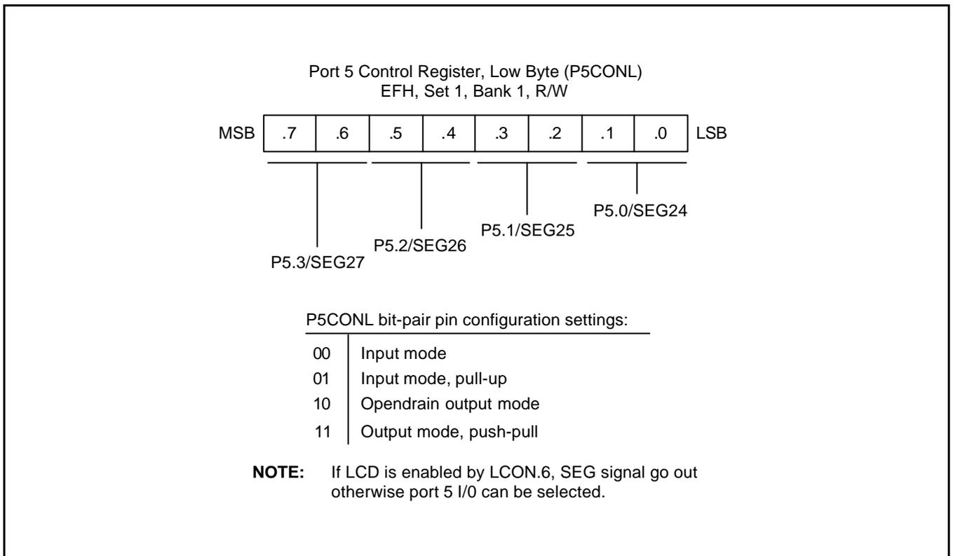
Figure 9-15. Port 5 Low-Byte Control Register (P5CONL)
