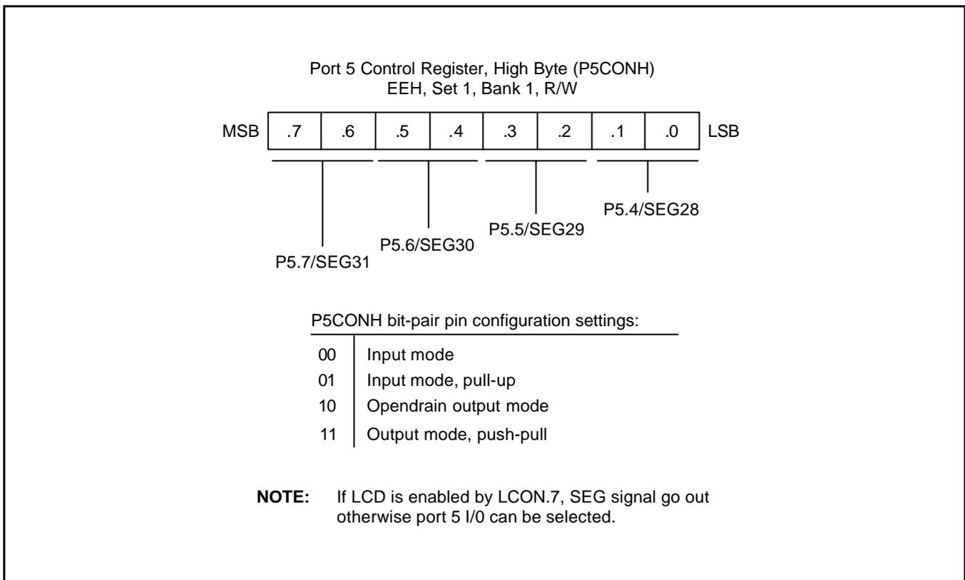
Figure 9-14. Port 5 High-Byte Control Register (P5CONH)
