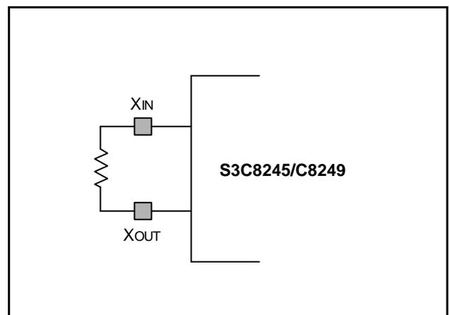
Figure 7-2. Main Oscillator Circuit
