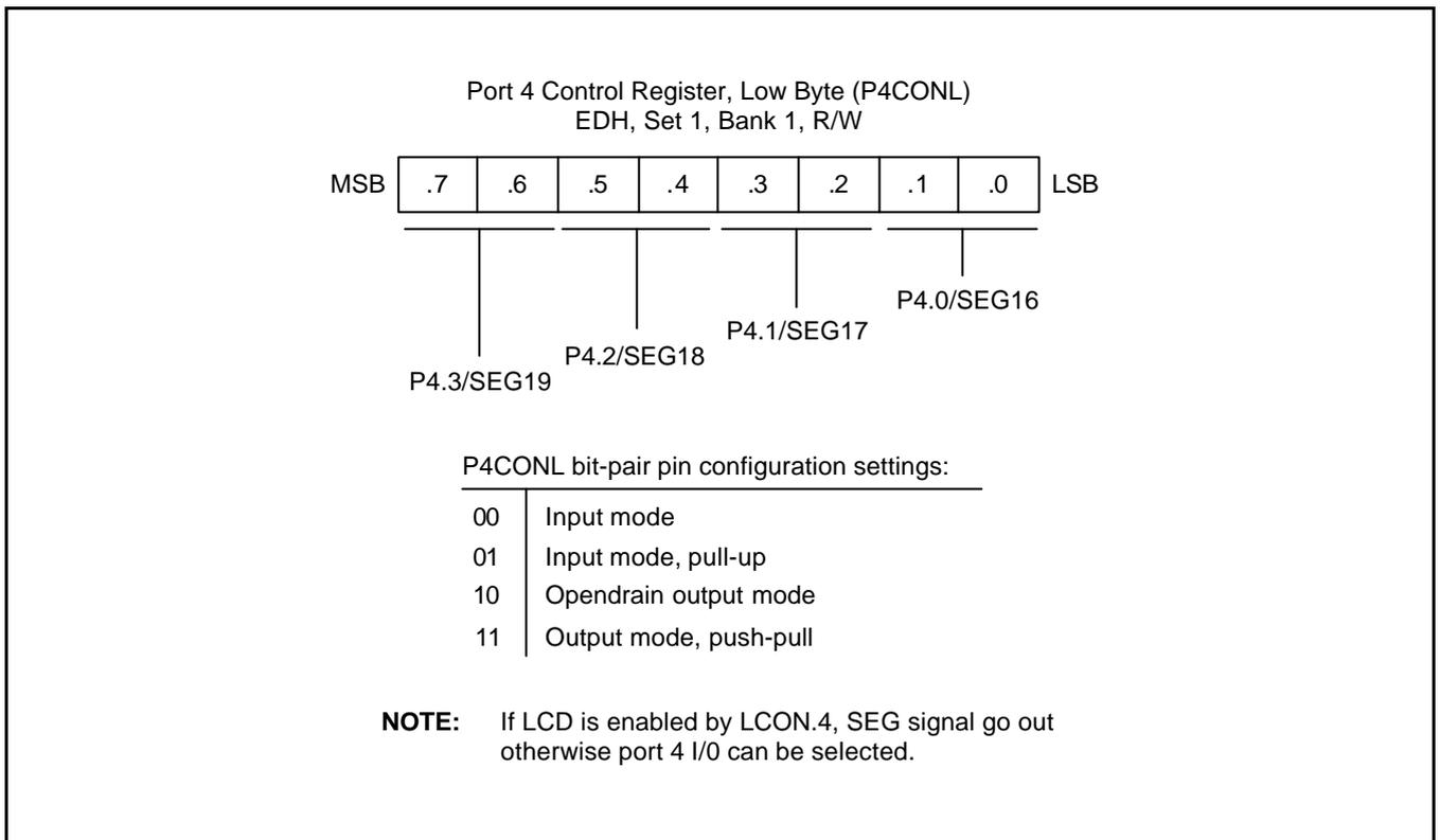
Figure 9-13. Port 4 Low-Byte Control Register (P4CONL)
