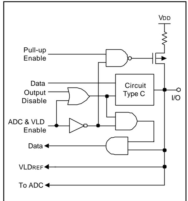
Figure 1-10. Pin Circuit Type F-18 (P2.7/VLD<sub>REF</sub>)
