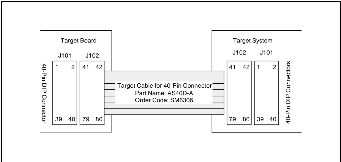
Figure 22-4. S3E8240 Cables for 80-QFP Package
