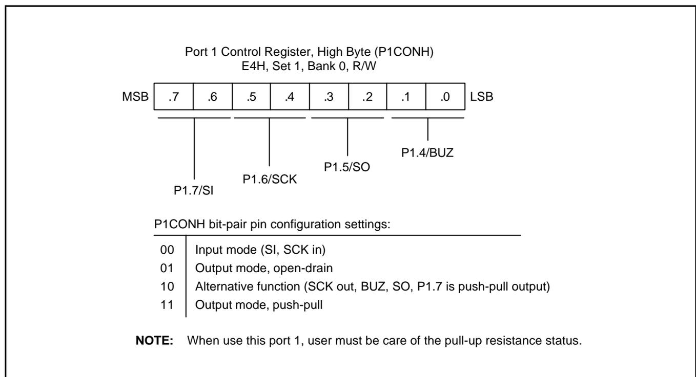
**Figure 9-5. Port 1 High-Byte Control Register (P1CONH)**
