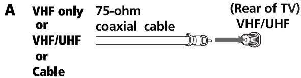
Use this to connect the TV to a cable system or an antenna with a 75-ohms cable.
