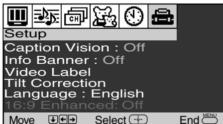
Select closed captioning options, display the name of the current program and its remaining time, label video inputs, adjust tilt correction (available only for KV-25FS120), select menu languages, or run a demo of the menus.
