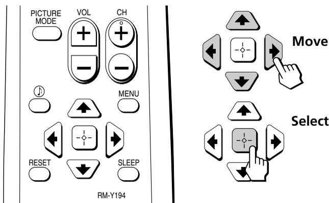
To navigate on the on-screen menus, use the “arrow” buttons (↑, ↓, ←, →) to move the cursor. Pressing these arrows will cause the cursor to move in the corresponding direction. Pressing center button (⊕) will allow you to select an option.
