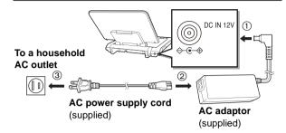
The unit is in the standby condition (the  $[\mathfrak{O}]$  indicator lights) when the AC power supply cord is connected. The primary circuit is always "live" as long as the AC adaptor is connected to an electrical outlet.
