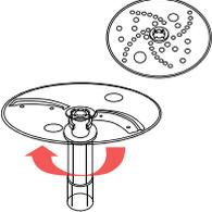
4. Once the Adapter is inserted into the Disk, rotate the disk until it is seated.
