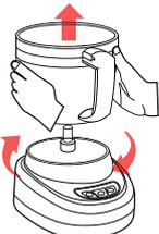
4. Rotate the Main Handle to the left until it is unseated and lift off of the motor housing.
