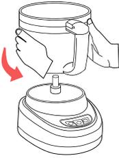
1. Place the large work bowl onto the motor housing with the main handle to the left of the power panel. This aligns the bowl to properly engage the safety interlock. Turn the main handle to the right until it “clicks” or “locks” into place. The main handle should now be centered with the Power Panel.
