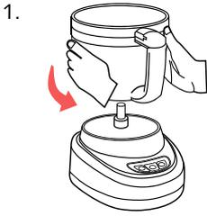
1. Place the large work bowl onto the motor housing with the main handle to the left of the power panel. This aligns the bowl to properly engage the safety interlock. Turn the main handle to the right until it “clicks” or “locks” into place. The main handle should now be centered with the Power Panel.
