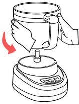
1. Place the large work bowl onto the motor housing with the main handle to the left of the power panel. This aligns the bowl to properly engage the safety interlock turn the main handle to the right until it clicks” or “locks” into place. The main handle should now be centered with the Power Panel.
