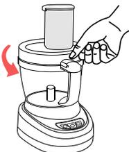
4. Place the Work Bowl Cover onto the Work Bowl with the interlock “tab” to the left of the main handle. Turn the Cover to the right until it “clicks” or “locks” into place. The “tab” should now be aligned with the Main Handle.
