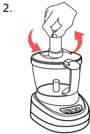
2. Place the Large Blade or Dough Blade onto the main motor shaft. You may have to rotate the blade partially to properly “seat” onto the shaft.
