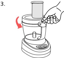
3. Place the Work Bowl Cover onto the Work Bowl with the interlock “tab” to the left of the main handle. Turn the Cover to the right until it “clicks” or “locks” into place. The “tab” should now be aligned with the Main Handle.
