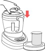
5. Place the Work Bowl Cover onto the Work Bowl with the interlock “tab” to the left of the main handle. Turn the Cover to the right until it “clicks” or “locks” into place. The “tab” should now be aligned with the Main Handle.
