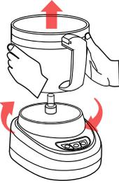
3. Rotate the Main Handle to the left until it is unseated and lift off of the motor housing.
