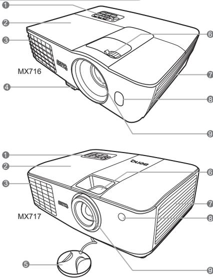
1. External control panel (See "Controls and functions" on page 10 for details.)
