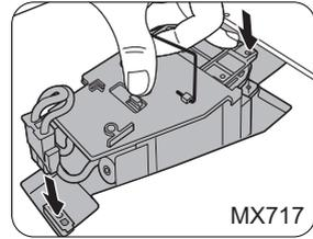
10. Tighten the screw that secures the lamp.
