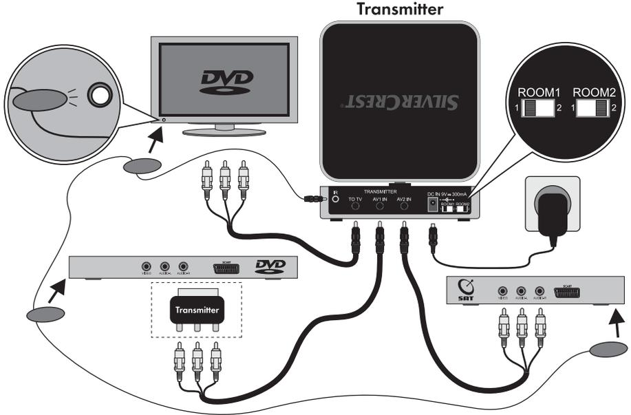
Fig. Connection example for Transmitter
