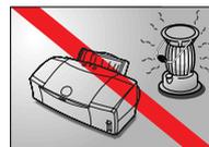
Set up and use the printer in a location where ambient temperature is within 5°C~35°C (41°F~95°F) and 10%~90% humidity with no condensation.
