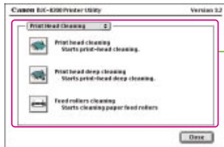
This dialog provides the selections for print head cleaning, printing test prints, and other maintenance tasks. Execute print head cleaning to correct poor print quality.
