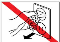
Never remove the power cord from the power outlet until you have switched the printer off by pressing the POWER button. After the POWER/ERROR lamp extinguishes, you can unplug the power cord from the power outlet.
