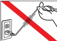
Pulling on the power cord could damage the cord and cause a fire or electric shock.
