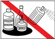
If a flammable solvent contacts an electrical component inside the printer, this could cause a fire or electric shock.
