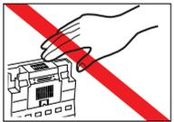
These metal parts become very hot during printing and could cause minor burns.
