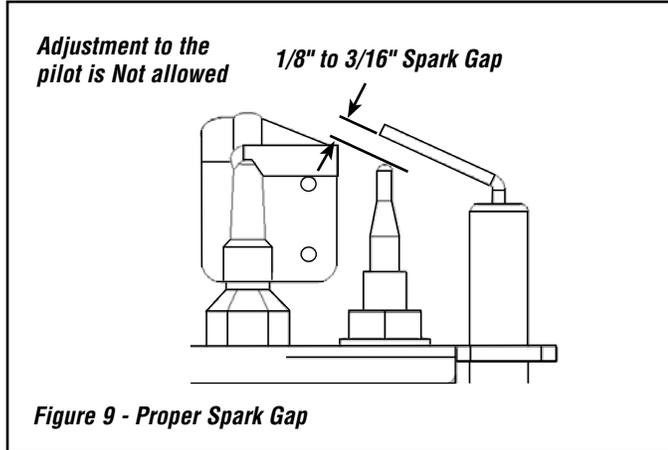
Figure 9 - Proper Spark Gap
