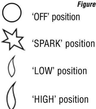
The control knob is located on the lower right hand side of the outer case. It is of a spherical design and is marked as shown in **Figure 19**.
