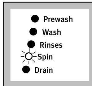
To select **Drain**, now press the SKIP button three times, the **wash - rinses - spin** LED,s go out and the **Drain** LED remains lit.
