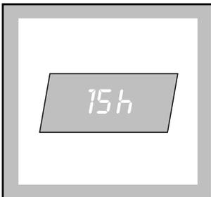
The delay time is displayed for 3 seconds, then the duration of the selected programme reappears. After you have pressed the START/PAUSE button, the countdown begins, and the delay time value decreases by one unit every hour. You can delay the start of every programme by up to 24 hours in one hour intervals selecting the DELAY START button.
