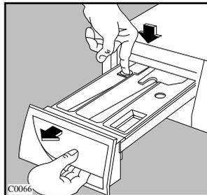
To facilitate cleaning, the top part of the additive compartment can be removed.
