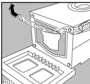
5. Set the machine upright and remove the remaining rear screw. Slide out the relevant pin.
