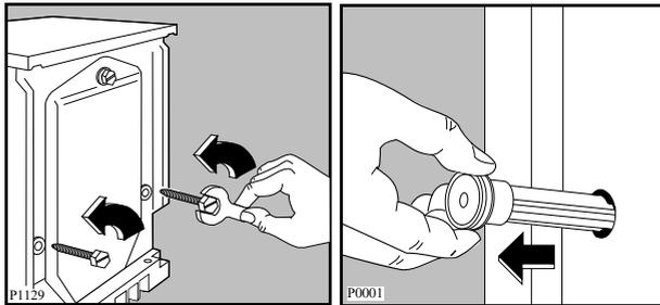
2. Remove the polystyrene block(s) from the bottom of the machine and release the two plastic bags.
