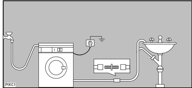
The drain hose may be extended to a maximum of 4 metres. An additional drain hose and joining piece is available from your local Service Centre.
