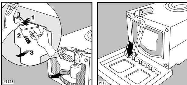
4. Very carefully slide out the right polythene bag, removing it towards the left and then upwards.
