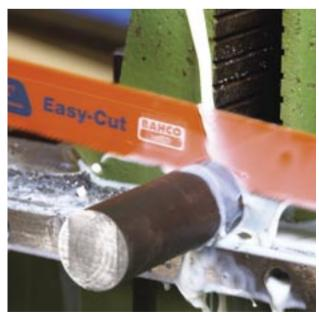
Easy-Cut cuts a variety of materials for instance mild steel, stainless steel and tool steel as well as non-ferrous materials including aluminium, copper, brass and even plastics.
