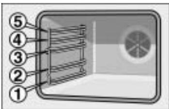
The shelf can be inserted at 5 different heights in the oven.
