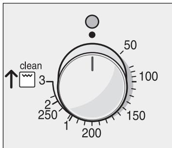
Use the temperature selector to set the temperature or grill setting.
