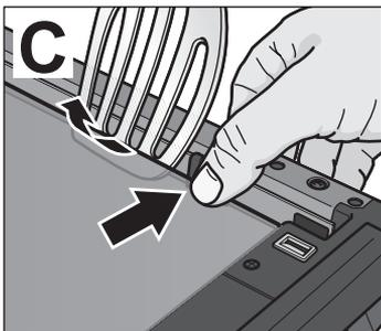
1. Press in the retaining clip with your thumb on one side and disengage the **inner door glass** e.g. with the spatula, then repeat on the other side. (Fig. C).
