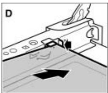
1. Push the glass panel back at an angle. (Fig. D).
