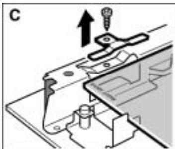
4. Unscrew the clips on the right and left and remove them (Fig. C).
