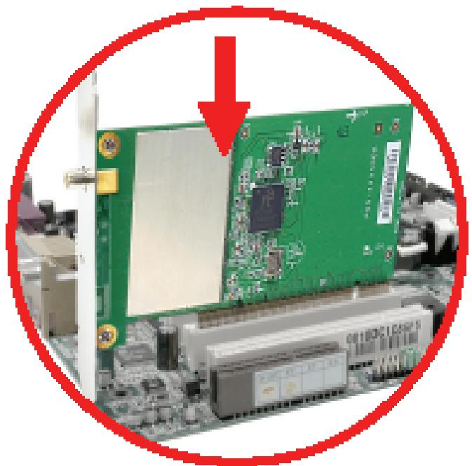
*DO NOT hold the wireless LAN adapter on the golden finger while installing; doing this may cause interference or damage.*
