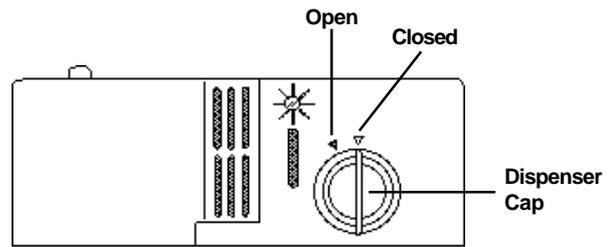
1. To open the dispenser, turn the cap to the “open” (left) arrow and lift it out.
