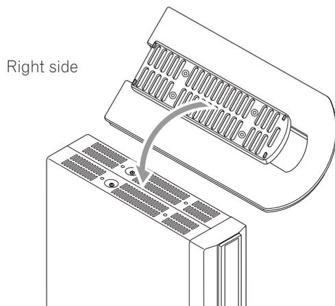
You can remove the shock absorbing pads.
