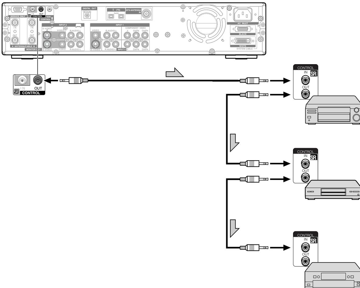
The control cables (commercially available) are mono sound cables with mini plugs (no resistance).
