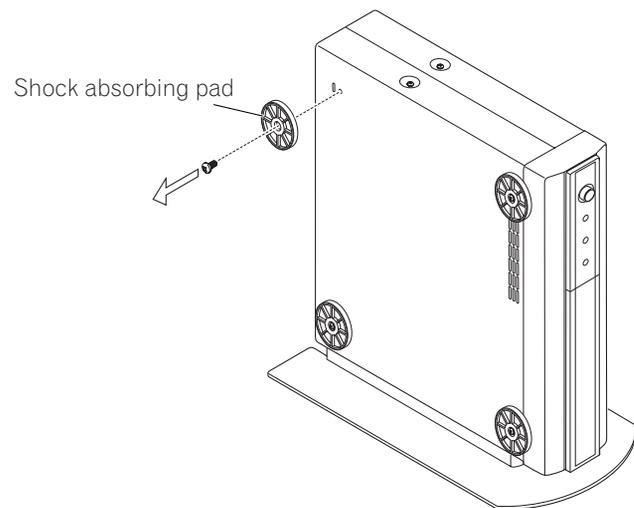
Keep the shock absorbing pads and screws. They are required when you place the Media Receiver in the horizontal position.
