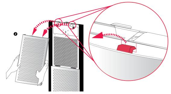
2 Lift finishing panel free of the dead front panel and remove.
