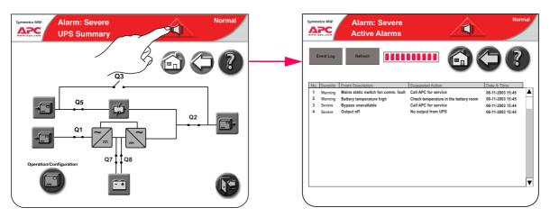
Press the red triangular alarm symbol to view active alarms. Only active alarms will appear on the screen. Pressing the alarm symbol will also mute audible alarms.
