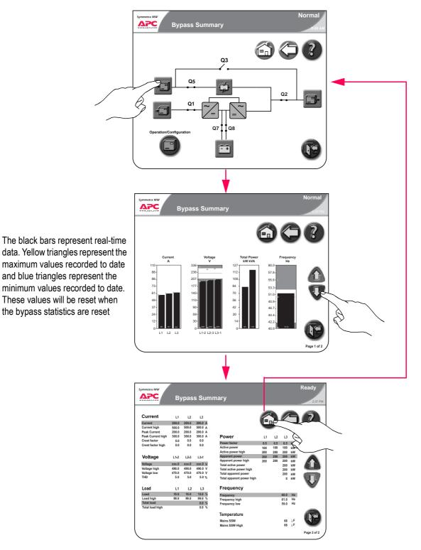
The two Bypass Summary screens provide status of voltage, power, current, frequency, etc.
