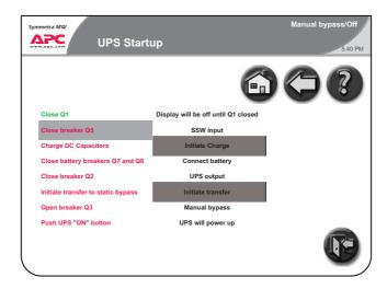
The UPS Start-Up screen shows a list of actions, which need to be completed in order to start up the UPS from Manual Bypass Operation. The actions are initially indicated in red to show that they have not yet been completed. A yellow bar will highlight the actions in the order in which they need to be completed. As actions are completed they will change to green.
