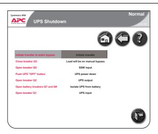
The UPS Shutdown screen shows a list of actions, which need to be completed in order to shut down the UPS. The actions are initially indicated in red to show that they have not yet been completed. A yellow bar will highlight the actions in the order in which they need to be completed. As actions are completed they will change to green.
