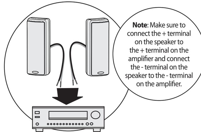
**Note:** Make sure to connect the + terminal on the speaker to the + terminal on the amplifier and connect the - terminal on the speaker to the - terminal on the amplifier.
