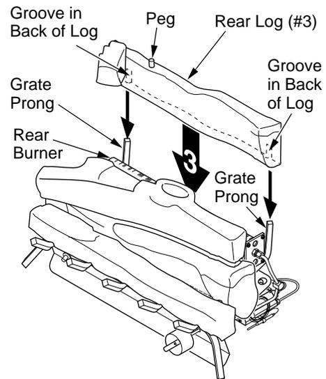
**Figure 23 - Installing Rear Log (#3) [18" Variable Manually-Controlled Set Shown]**
