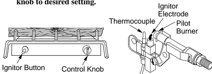
Figure 27 - Control Knob and Ignitor Button Location
