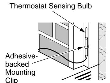
**Figure 44 - Locating Thermostat Sensing Bulb on Factory-built Metal Fireplace**
