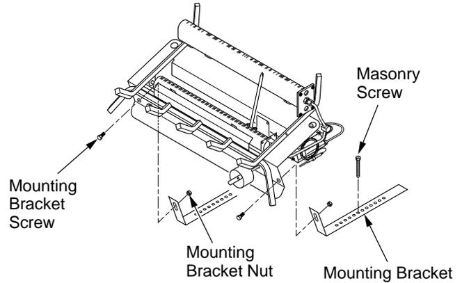
**Figure 13 - Attaching Heater to Fireplace Floor (Variable Manually-Controlled and Thermostatically-Controlled Models Only)**
