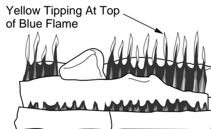
**Figure 37 - Incorrect Front Burner Flame Pattern**
