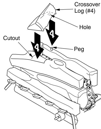
**Figure 24 - Installing Crossover Log (#4) [18" Variable Manually-Controlled Set Shown]**
