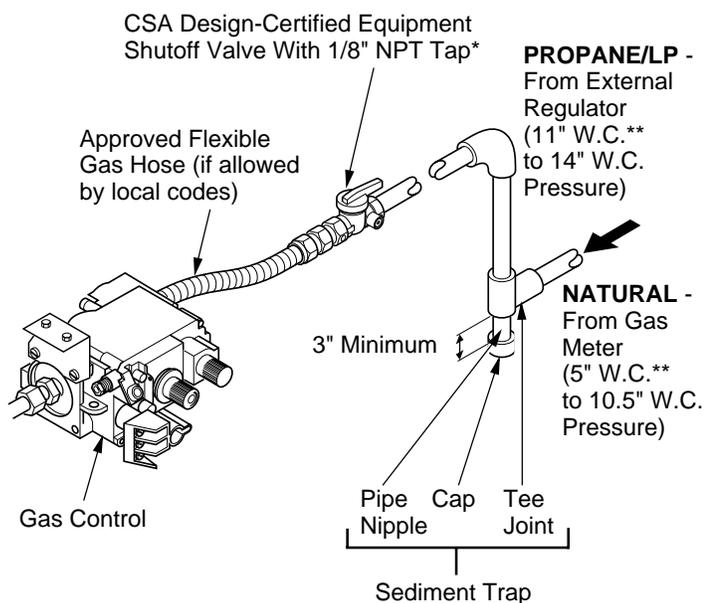
**Figure 17 - Gas Connection (Remote-Ready Models Only)**
