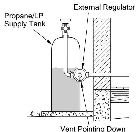
Figure 15 - External Regulator With Vent Pointing Down
