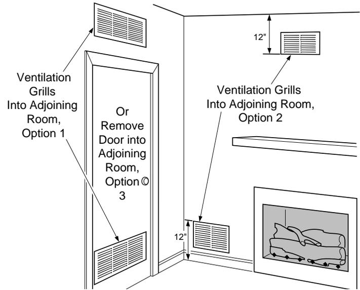
Figure 2 - Ventilation Air from Inside Building
