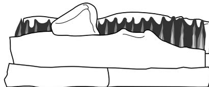
**Figure 36 - Correct Front Burner Flame Pattern**
