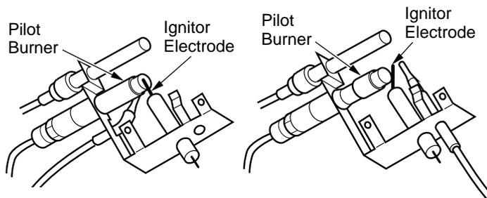
Figure 30 - Pilot (Propane/LP) Figure 31 - Pilot (Natural)
