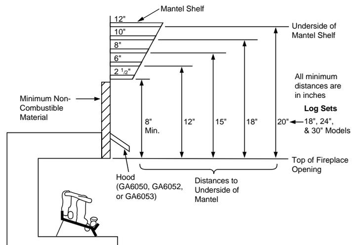
Figure 7 - Minimum Mantel Clearances When Using Hood
