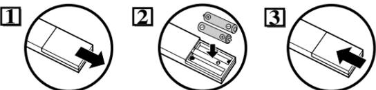
Install two AAA batteries (supplied) matching the polarity indicated inside battery compartment of the remote control.
