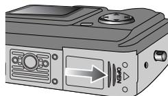
2. Insert the card all the way into the card slot. The card pins and the LCD monitor should face in the same direction. The card will be fitted.
