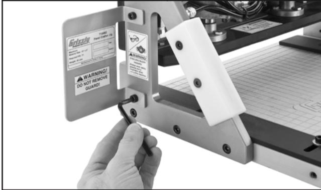
**Figure 4.** Attaching guard to jig.
