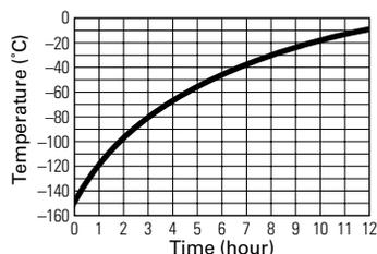
LN<sub>2</sub> back up system operation characteristics
