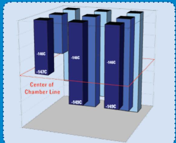
Comparison of temperature distribution in a liquid nitrogen freezer (vapor phase) and SANYO's MDF-C2156VANC mechanically refrigerated cryogenic freezer. Graph shows temperatures at different locations within the chamber. This data demonstrates that 100% of the MDF-C2156VANC storage space maintains uniform storage temperatures safely below -130°C, while temperature in LN<sub>2</sub> vapor system is dependent on storage location.
