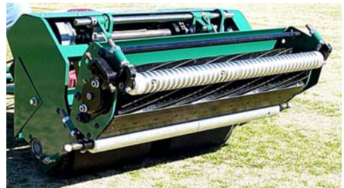
GT can be pivoted back for easy turning and direction changes.
