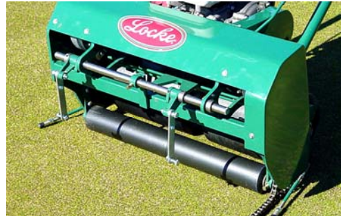
Support Roller provides full float action of cutting units and aids in stripping
