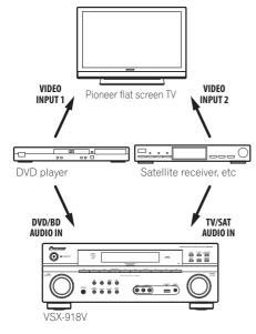
To make the most of the SR+ features, you should connect your source components (DVD player, etc.) in a slightly different way to that described in this chapter. For each component, connect the video output directly to the flat screen TV, and just connect the audio (analog and/or digital) to this receiver.
