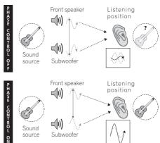
Phase Control technology provides coherent sound reproduction through the use of phase matching <sup>1</sup> for an optimal sound image at your listening position. The default setting is on and we recommend leaving Phase Control switched on for all sound sources.
