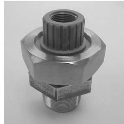
The Insertion Adapter mounts Model 399VP into a 1-1/2 inch NPT process pipe. Unscrewing the hex nut allows easy sensor removal without twisting the sensor cable.
