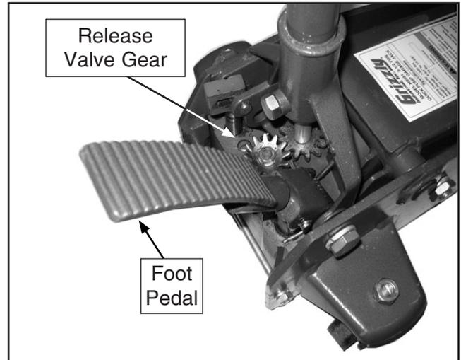
Figure 2. Pump pedal and release valve gear.
