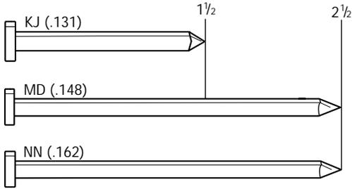
8-10 Gauge. 1<sup>1</sup>/<sub>2</sub>" - 2<sup>1</sup>/<sub>2</sub>" 4d - 8d. Full Round-Head Nails. Bright Basic and Hot Dip Galvanized Nails. Capacity 30.
