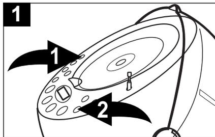
Press the POWER button ❶ to turn the unit on. Press the FUNCTION button ❷ until radio is selected.
