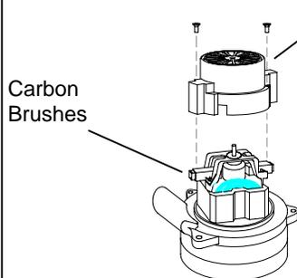
If armature commutator is grooved, extremely pitted or not concentric, the motor will need to be replaced or sent to a qualified service center.
