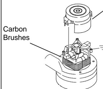
**Note:** When replacing carbon brushes loosen wire terminal **BEFORE** removing screws on bracket.
