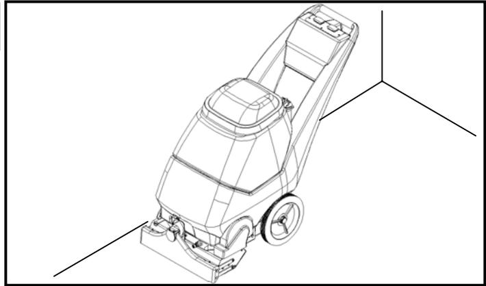
After cleaning, turn off all controls, return brush to storage position and carefully unplug machine.
