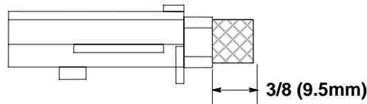
Periodically check the length of the carbon brushes. Replace both carbon brushes when either is less than 3/8" (9.5mm) long.
