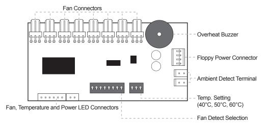
Fan1 to Fan8 could be set either "ENABLE" or "DISABLE". When all the fans are set on "DISABLE", the Fan LED will have no light on.
