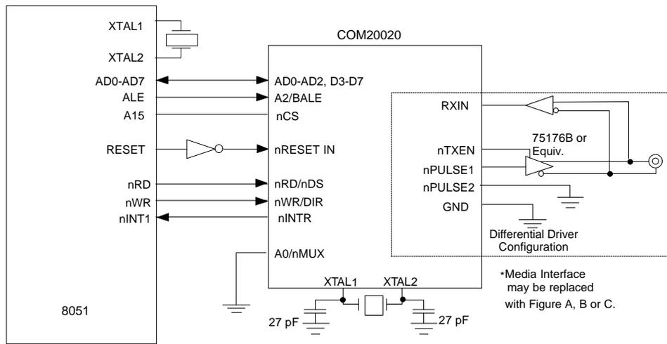
FIGURE 2 - MULTIPLEXED, 8051-LIKE BUS INTERFACE WITH RS-485 INTERFACE
