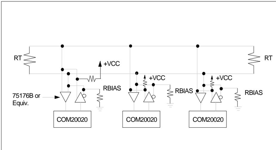
FIGURE 4 - COM20020 NETWORK USING RS-485 DIFFERENTIAL TRANSCEIVERS
