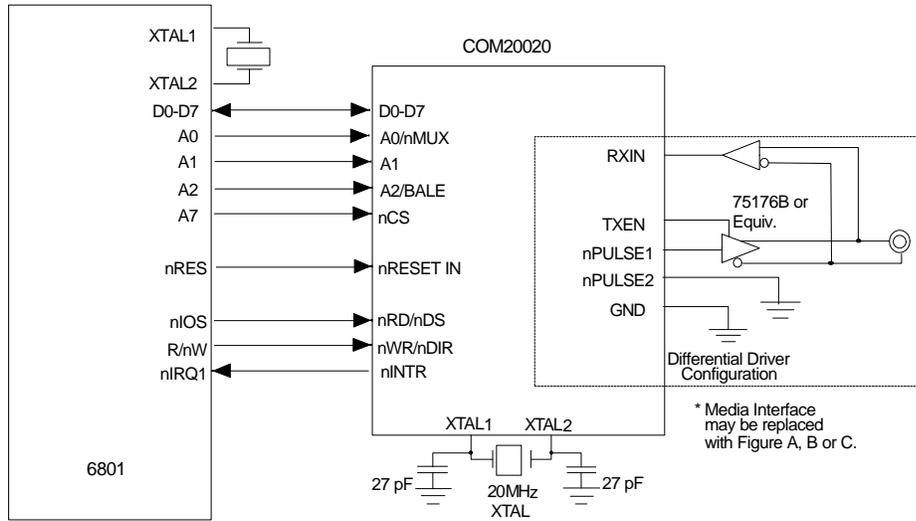
FIGURE 3 - NON-MULTIPLEXED, 6801-LIKE BUS INTERFACE WITH RS-485 INTERFACE
