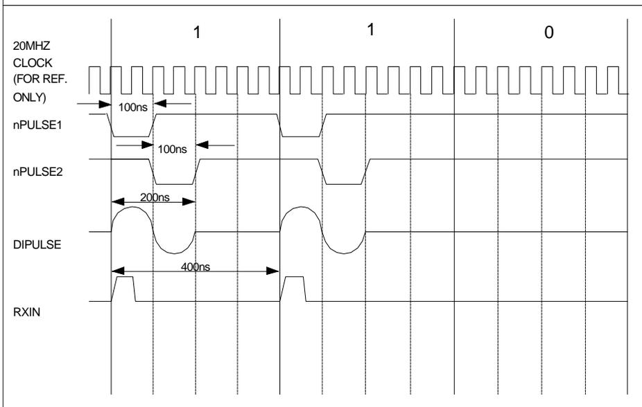
FIGURE 5 - DIPULSE WAVEFORM FOR DATA OF 1-1-0
