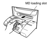
When an MD is inserted, the front panel closes automatically.
