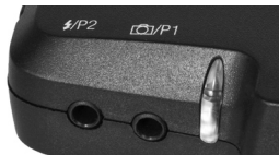
Use 1/P2 for remote manual flash
