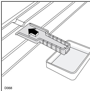
3. when defrosting is completed, dry the interior thoroughly and refit the plug; keep the scraper for future use;
