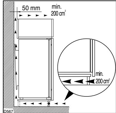
For safety reasons, minimum ventilation must be as shown in Fig.
