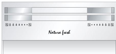
Regulation for each drawer is separate and is controlled using the slide valve at the front of the drawer.
