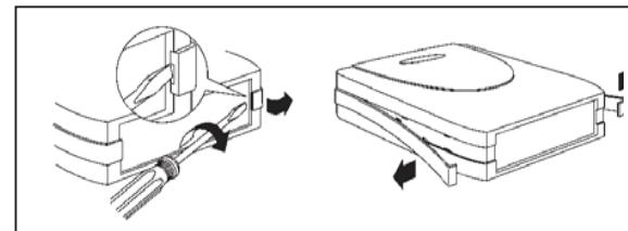
Carefully prise the two fixing rails from the backside of the housing using a screwdriver. Strip the rails off carefully from back to front. Separate the top cover from the base.
