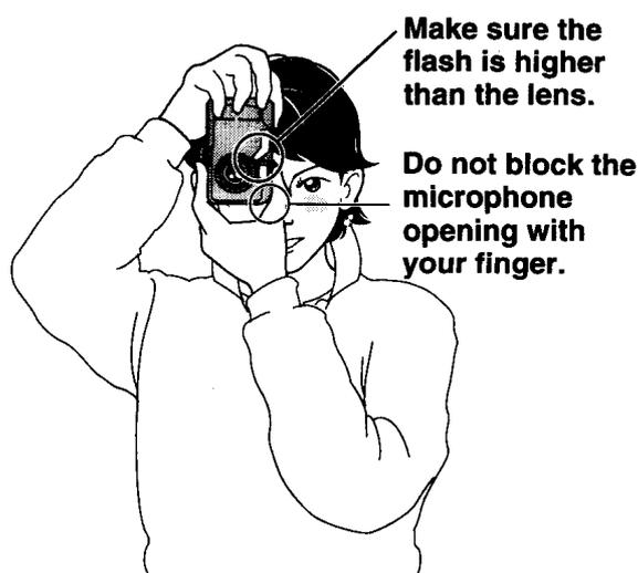
Make sure that the flash or the lens are not blocked by a finger or the hand-strap.
